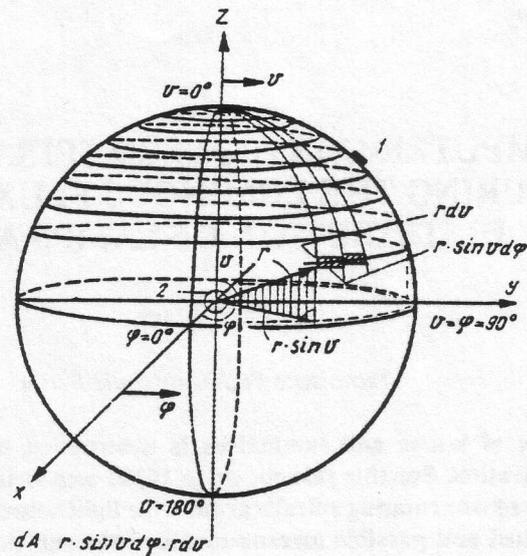
Fig. 1. Principle of spiral scanning: 1) photodetector; 2) light source.
