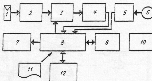
Fig. 5. Microcomputer-controlled electronic integration of luminous flux. 1) Sensor; 2) Input amplifier; 3) Sample and Hold circuit; 4) Analog/Digital Converter; 5) I/O; 6) Positioning indicator; 7) Printer; 8) Microcomputer; 9) Rapid arithmetic processor; 10) Power supply; 11) Programme; 12) Monitor with keyboard.
